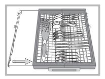
The third basket is equipped with two sliding side trays to make the most of the height of the space below. The upper rack can be adjusted for height based on requirements: high position to place bulky crockery in the lower rack and low position to make the most of the tip-up dispensers/ sectors by creating more space upwards.
